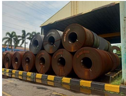
Gambar 1 HRC (Hot Rolled Coil)
