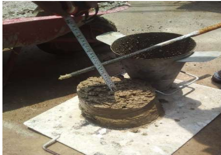
Test Slump Beton Cair
