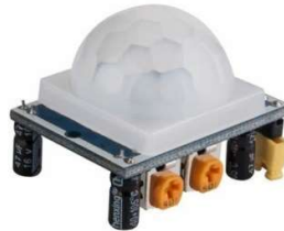
Gambar 2.2. Sensor Passive Infrared (PIR)
