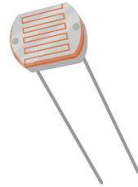
Gambar 2.3. Sensor Light Dependent Resistor (LDR)
