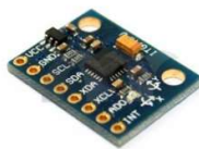
Gambar 2.4. Sensor Inertial Measurement Unit (IMU)
